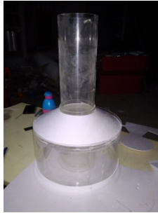
Polycarbonate pressure tank for underwater sea research
