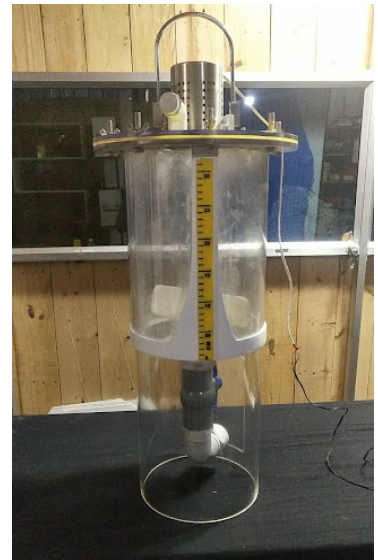
Polycarbonate Reactor for Medicine research
